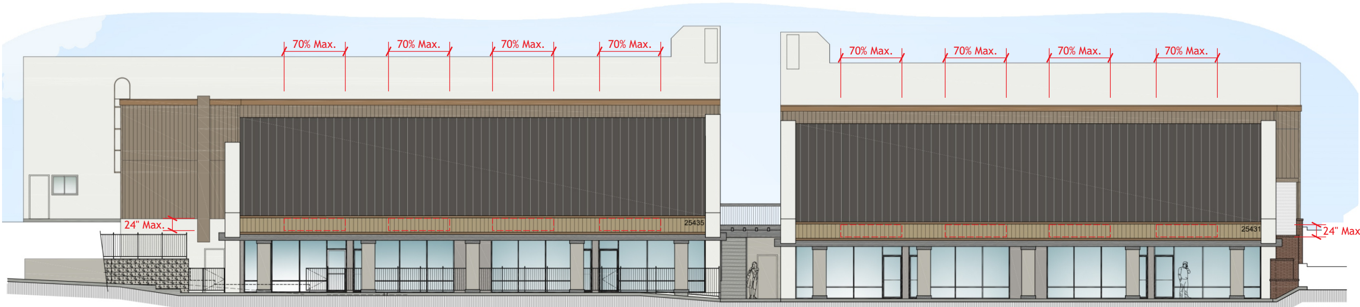
TENANT SIGNAGE LOCATIONS (NORTHWEST ELEVATION)
