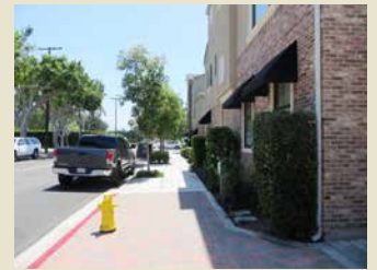
A street furniture/buffer zone, a pedestrian through zone and frontage zone, East 3rd Street, Tustin
