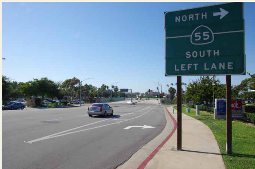
Sign indicating access to the I55, Costa Mesa; the signage is positioned so it is clearly visible for drivers, but high enough for pedestrians to pass under, and the posts are positioned so that the sidewalk is relatively unobstructed
