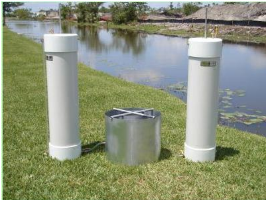
Figure VII.10. Double Ring Infiltrometer Set-up with Mariotte Tubes
