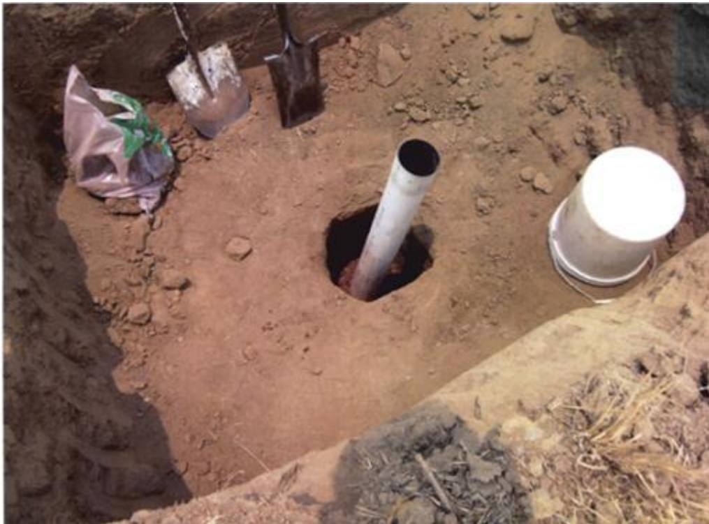
Figure VII.17. Photo of Percolation Test Pit.
