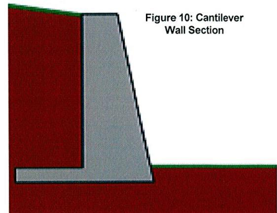
levered base is reinforced and is designed to prevent uplifting at the heel of the base, making the wall strong and stable. Reinforced concrete cantilevered walls sometimes have a batter. They can be faced with stone, brick, or simulated veneers. Their front faces can also be surfaced with a variety of textures. Reinforced concrete cantilevered walls are typically poured in place using forms. When the use of forms is not desired, reinforced concrete block cantilevered walls are an option.
