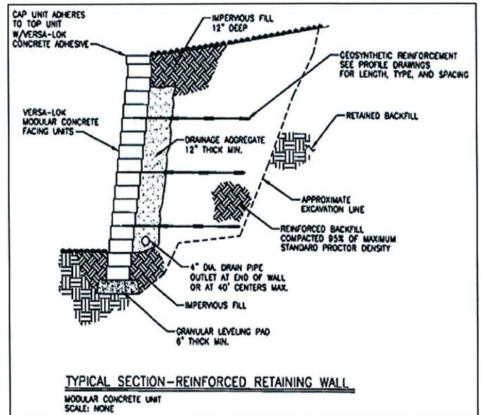
Figure 12: MSE Wall Construction
